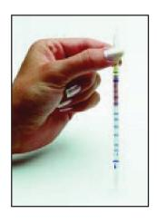
Cross contamination, from test to test, is eliminated through one time use of individual components. The components are premeasured to ensure accurate results in parts per million. In addition, no temperature correction is needed from 41°F to 176°F. Use this innovative product confidently with any abrasive.
