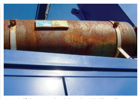
ABOVE A If flash rust occurs on the steel substrate, the steel should be tested for contamination, because the rust is probably the result of non-visible soluble salt contamination. Without some ionic species present, there will not be rust. Even very low soluble salt levels can cause an appreciable amount of flash rust.
