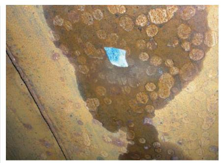
**ABOVE** Often a coatings specification for a steel substrate will call for surface prep using Ultra High Pressure Water Jetting (UHP-WJ). However, salts that have attached to and reacted with a metal substrate sometimes cannot be removed even with 40,000 psi UHP-WJ. Once these chloride ions form an attachment to the metal substrate, a very high level of energy is necessary to break that electro-chemical bond.
