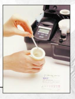
The CHLOR\*TEST "CSN Salts" uses a unique patented extract solution, CHLOR\*EXTRACT™, to retrieve surface salt contamination. This special extract enhances retrieval rates, thereby increasing accuracy. The greater the retrieval rate, the more accurate the test results.
