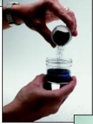
CHLOR\*TEST "A" uses ASTM D4940 principles, but offers the additional value of chloride ion specific measurement.
