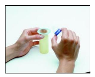
I Empty the entire contents of the CHLOR\*EXTRACT™ container into the CHLOR\*SLEEVE™. Peel off the protective backing, pinch the sleeve to expel some of the air and adhere the sleeve to the surface to be tested.
