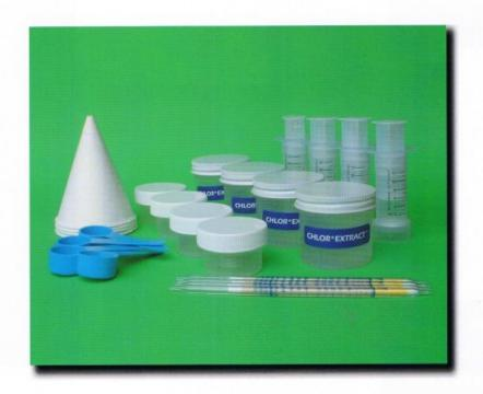
An easy to use, accurate field test for chloride contamination in concrete
