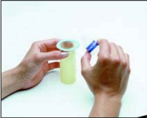
**1** Empty the entire contents of the CHLOR\*EXTRACT™ container into the CHLOR\*SLEEVE™. Peel off the protective backing, pinch the sleeve to expel some of the air and adhere the sleeve to the surface to be tested.
