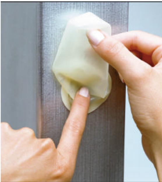
The CHLOR\*TEST "CSN Salts" uses a unique patented extract solution, CHLOR\*EXTRACT™, to retrieve surface salt contamination. This special extract enhances retrieval rates, thereby increasing accuracy. The greater the retrieval rate, the more accurate the test results.
