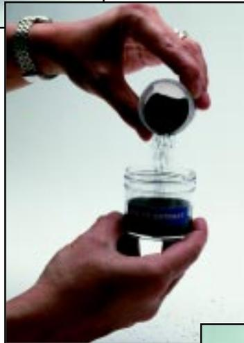
CHLOR\*TEST "A" uses ASTM D4940 principles, but offers the additional value of chloride ion specific measurement.
