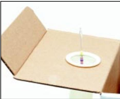
**3** Snap the sealed ends off the glass tube, insert it into the sleeve and down into the extract. In about two minutes read the color change to identify the chloride level in both parts per million and micro grams per centimeter squared, the ratio is 1:1.
