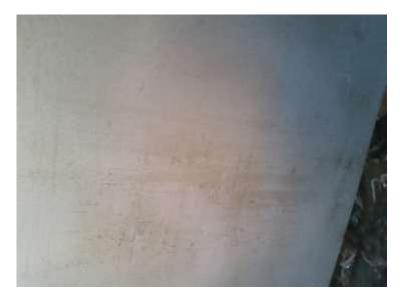
Areas that flash rusted were reblasted on April  $1^{st}$ . 12 hours later reblasted areas had failed again:
