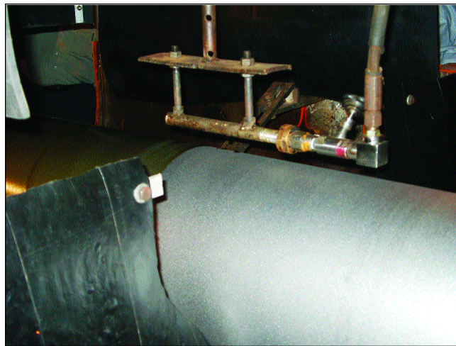
Fig. 4: Application of chromate treatment to profiled pipe
