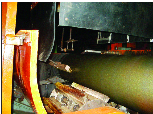
Fig. 5: Another view of application of chromate pretreatment to profiled pipe
