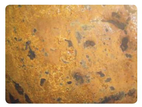
FIGURE 3 Corrosion on the inside of the produced water tank.
