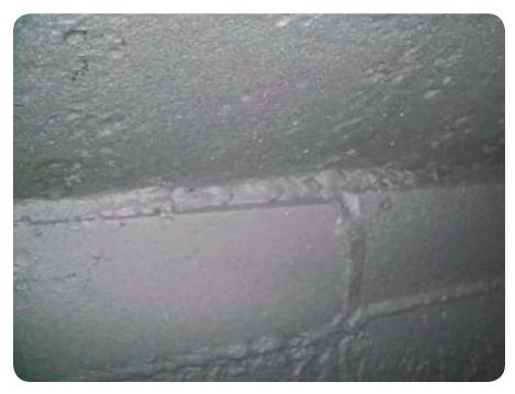
FIGURE 4 White metal blast, as defined in NACE No. 1/SSPC-SP 5.
