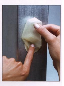
3 Snap the sealed ends off the glass tube, insert it into the sleeve and down into the extract. In about two minutes read the color change to identify the chloride level in both parts per million and micro grams per centimeter squared, the ratio is 1:1.
